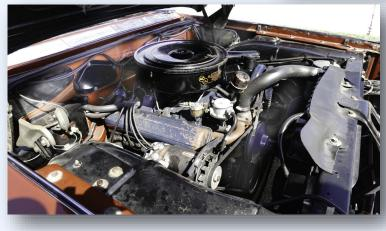
The cast iron 90 degree 6.4 liter engine is an 8 cylinder, overhead valve naturally aspirated engine with 2 valves per cylinder and a 4.0' bore and a 3.87" stroke, with a 10.5-1 compression, mounting a carter 4bbl carburetor or Rochester 4 -bbl downdraft Quadrajet. Transmission is a 4speed <u>Hydra-Matic (Jet-away)</u>. Neil is adding factory air.
