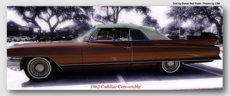
Engine: 390 cu in, 8.75 comp ratio, 325 hp, 404 ft-lb torque Wheelbase: 129.5", length 222", weight 4,625 lbs Performance: 0-60 mph @10.1 secs, ¼ mile @ 84 mph in 17.6 second top speed 122—124 mph Production: 16,800, first year of the dual master cylinder braking system Pompeian Red/White
